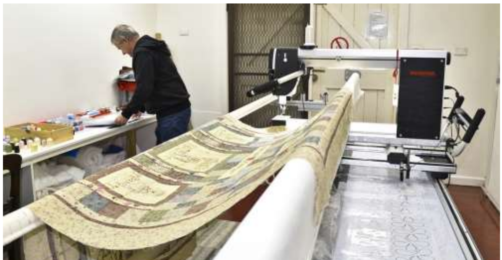
The impressive Bernina Q24 Long Arm quilting machine is able to accommodate large items and can sew up to 2,200 stitches per minute. Neil calculated that the project displayed on the frame would take up to 15 hours of customized work to reach completion, instead of the rigorous work associated with hand stitching the item.
